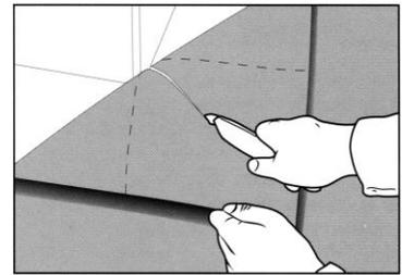
When fitting an out-corner, the sheet is folded against the corner and cut about 5 mm ( 1/4 in.) from the floor. The guidelines in the picture show the corner on the sheet and the position of the cut at about a 45-degree angle. Then a diagonal cut is made as shown.
