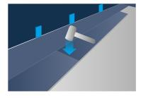
This method is then used to install all of the other rows. Make sure that the end joints are offset by at least 30 cm in the individual rows in order to achieve the best installation. To install the last row, the distance between the wall and the row installed is measured and transferred to the panel. The last row installed should be as close to half a panel's width as possible. Remember the 6 mm wide expansion joint.
