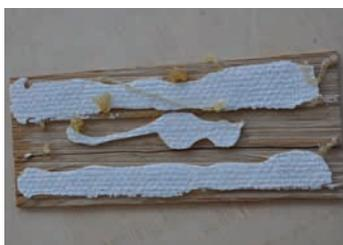
Adhesion test with a wall test sample
